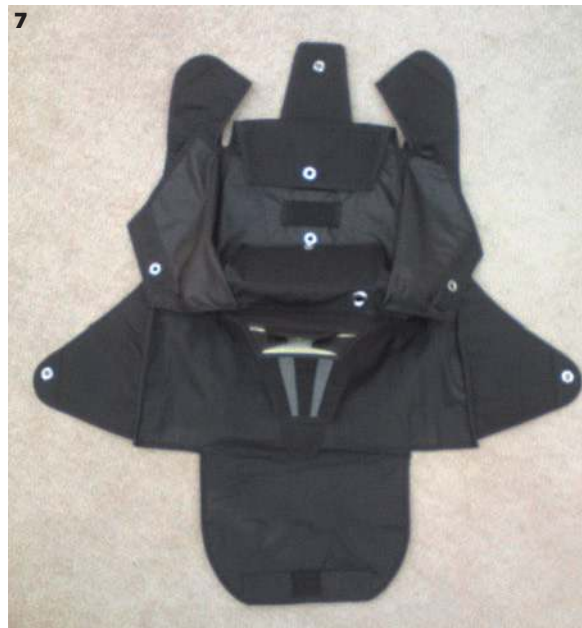
7-8 Reserve tray and centre piece sewn together, which are also sewn to the main tray
