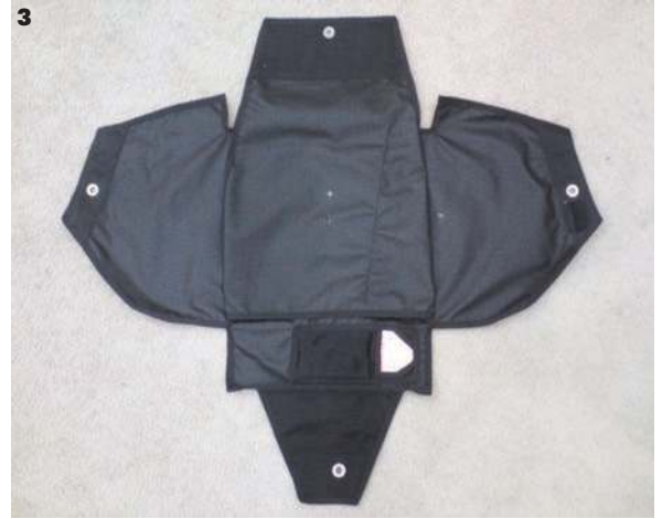
3 Reserve tray complete. The bottom flap is the main's top flap. The reserve tray bottom flap is actually part of the 'pretty centre piece' in photo 1 and will get added to the system during final assembly. You can also see the AAD pocket and cutter cable channel here
