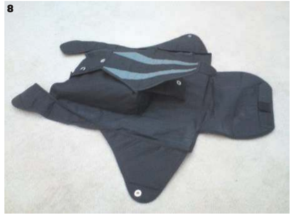
6 All the main components complete and laid out (except the main deployment system and the reserve freebag and pilot chute) There's probably around 323 individual pieces in the rig. The time taken to get here is around 121 hours of logged work
