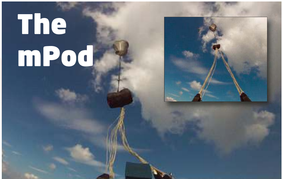
Video deployment footage of the mPod shows the lines paying out straight upwards, with no S-ing of the bag from side to side, as is inevitable with bungees
