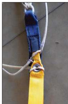
✗ Setting loop is above guide ring
