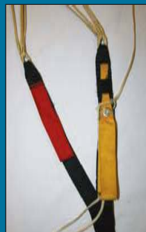
✗ Loop of excess brake line
