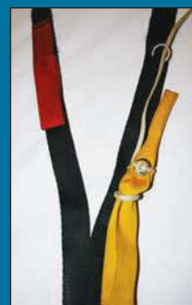
✗ Excess loop of line trapping toggle to riser
