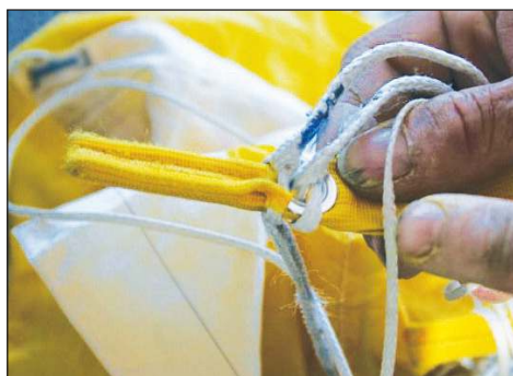
This worn toggle caused a malfunction
