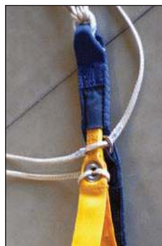
✓ Setting loop is below guide ring
