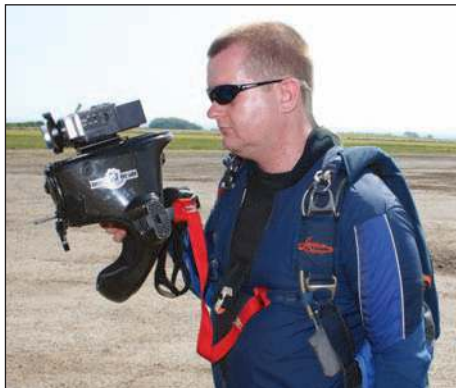
Woody demonstrates a camera restraint made from a simple piece of webbing
