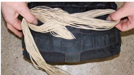
The mPod mouthlock is sealed by a flap containing a row of magnets, then the lines are S-folded on top of the bag
