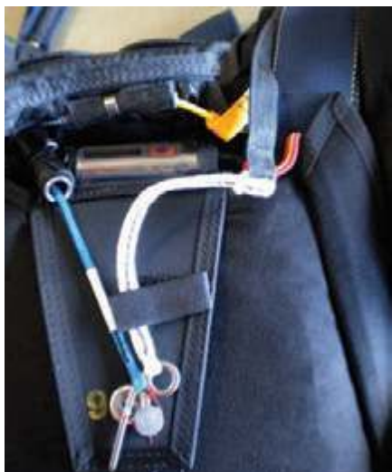
The Skyhook incorporates the reserve pin, and the reserve ripcord loops around that. The yellow Collins' Lanyard goes around the yellow cutaway cable
