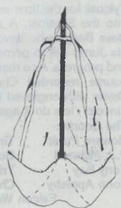
Fig. 4 Pilot Chute past its best - hem distorted.
