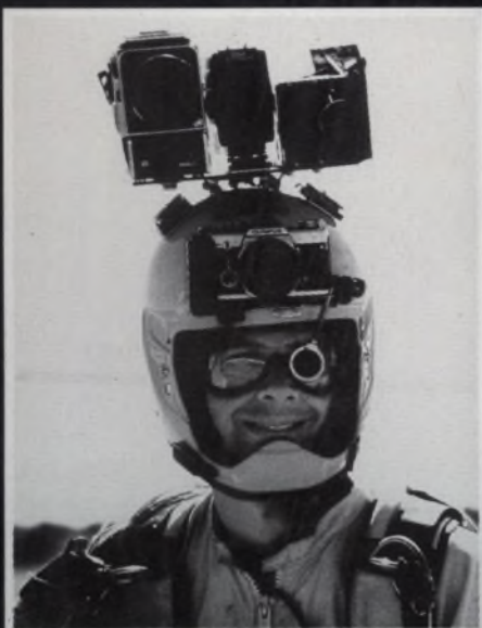
Photographer Norm Kent complete with freefall camera rig which includes a Hasselblad, Hitachi Video, an N9 16mm cine camera and an Olympus OM2 still camera. Total all up weight 26lb.
