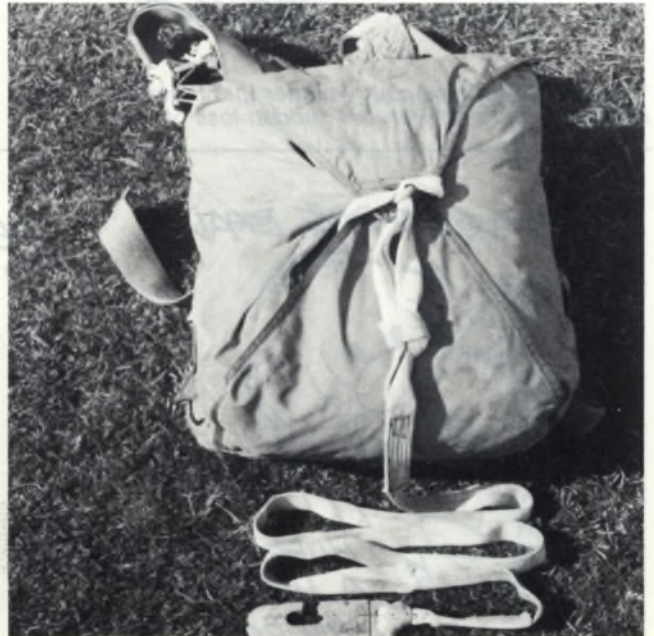
How the incorrect connecting of a static line caused a total malfunction and hang up.
