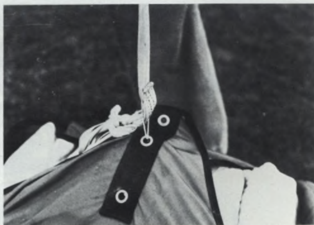
These two photographs illustrate a deployment sequence that ended in a total malfunction because the nylon loop snagged around the stitching on the bridal cord.
