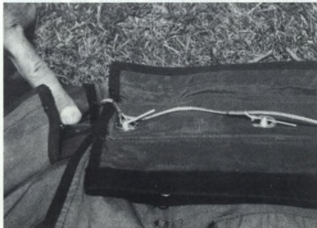
Bent pins are not a new disease. They can be cured by nylon loops.
