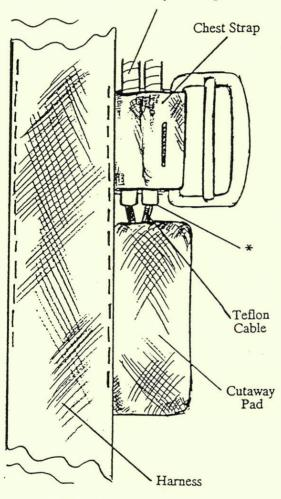
The BPA has been informed of a number of cut-away teflon cables that are being damaged by a poor finish to the inside of the cable housing near to the cutaway pad\*. Which can result in a hard pull.
