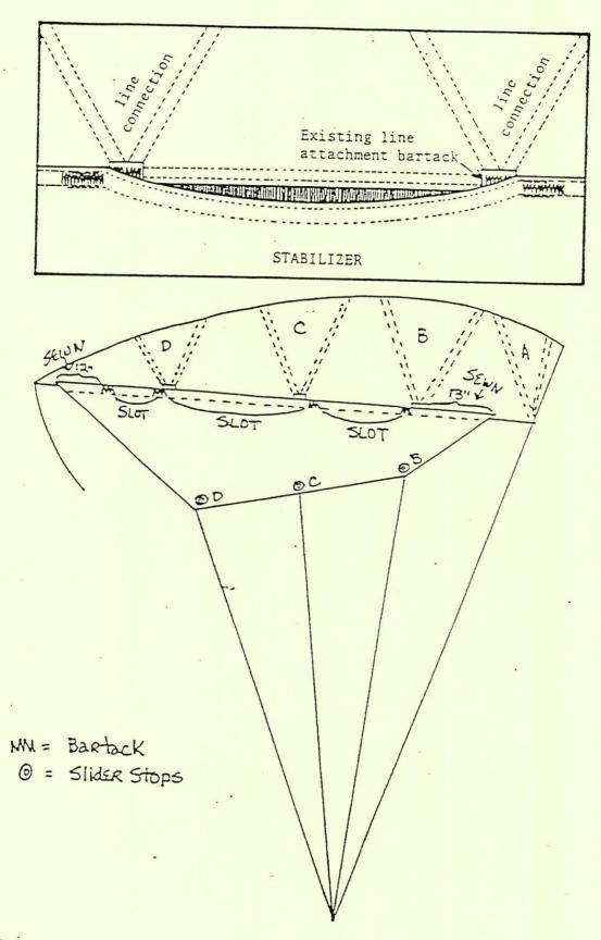
Because it is necessary to disconnect portions of the stabilizers adjacent to the "B" and "C" line attachment point to do this reinforcement, I have included this Diagram of stablizer configuration.
