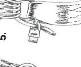
Pass the loop end thru the tab end, as shown.
