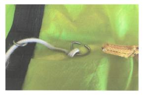
The left steering toggle was also attached in the same manner and it was found to have signs of stress and was close to detaching. During further inspection it was also discovered that two of the rapide links were found to be loose but were still closed. The equipment was made safe for further jumping by replacing the steering toggles and tightening up the connector links.
